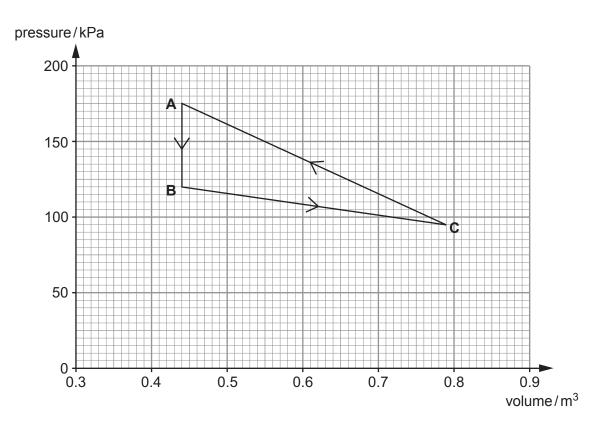
(a) There are **28.9 mol** of gas. The temperatures of points **A** and **B** are 321 K and 220 K respectively.
