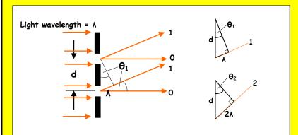
The light waves travelling along direction 1 interfere constructively to give the **Ist ORDER MAXIMUM**. For this to happen, the PD for light waves from adjacent slits = 1 A.
