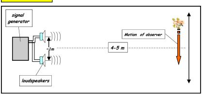
Two loudspeakers are connected to a single signal generator as shown in the diagram. The sound waves emitted by each speaker are then of equal frequency, wavelength and amplitude. An interference effect due to the superposition of the sound waves is observed in the region in front of the speakers.
