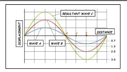
The <u>PRINCIPLE OF SUPERPOSITION</u> of waves states that when two or more waves meet at a point, the resultant displacement is the sum of the displacements of the individual waves.
