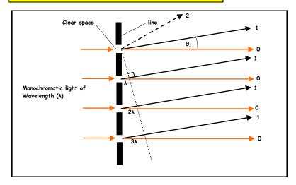
The above diagram shows a small section of a diffraction grating on which monochromatic light of wavelength  $(\Lambda)$  is normally incident. Consider what happens after the light passes through the grating.
