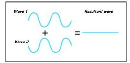
At points in between, the waves are somewhere in between being IN PHASE and ANTIPHASE and so the sound level heard is somewhere between LOUD and QUIET.
