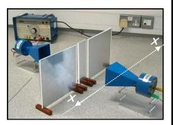
A microwave receiver connected to a microammeter is moved along a line XX,
