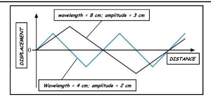
The diagram above shows two triangular waves. One of the waves has a wavelength of 8 cm and an amplitude of 3 cm, while the other has a wavelength of 4 cm and an amplitude of 2 cm.
