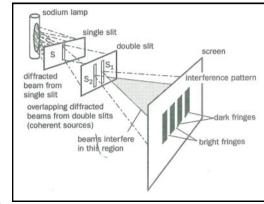
light source and it illuminates the narrow slit (S). Diffraction at S causes a diverging beam of light to fall on the two narrow slits  $S_1$  and  $S_2$  which are very close together and parallel to S. Since they are derived from a single source S, the two slits act as **coherent** light sources.
