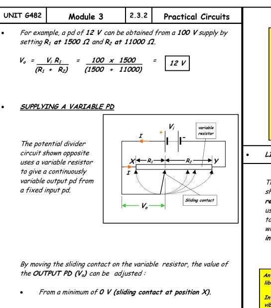
• To the maximum value when it is equal to the INPUT PD  $(V_i)$  (sliding contact at position Y).
