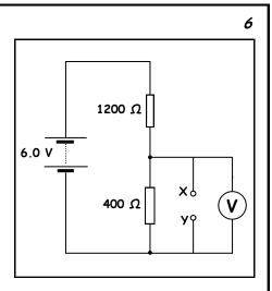
(i) Show that the voltmeter reading is 1.5 V.
