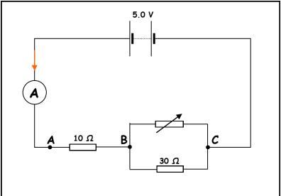
(a) The variable resistor is set on its maximum resistance of 20  $\Omega$ .
