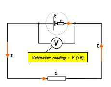
This is because when there is a current through the cell, some of its energy is converted into heat by the cell's internal resistance.
