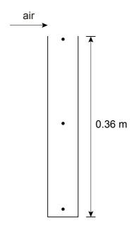
The length of the tube is 0.36 m. The air column in the tube is sounding its lowest (fundamental) frequency note.
