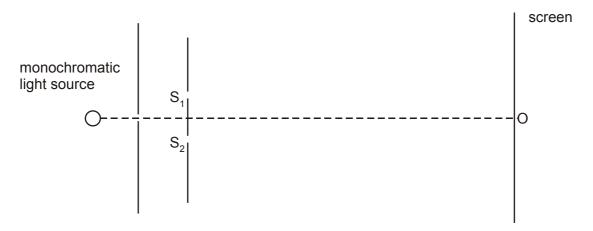
In a darkened room, a double slit (S<sub>1</sub>S<sub>2</sub>) is placed in front of a narrow single slit situated in front of a monochromatic (one frequency only) light source.
