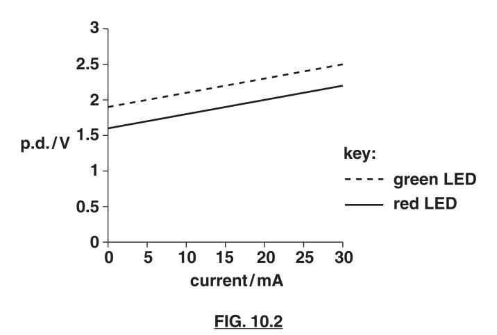
(i) Describe a difference shown in the graphs between the behaviour of the red and green LEDs.
