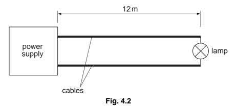
The lamp is rated at 24W, 6.0V. The power supply has negligible internal resistance and its output is adjusted so that the potential difference across the lamp is 6.0V.
