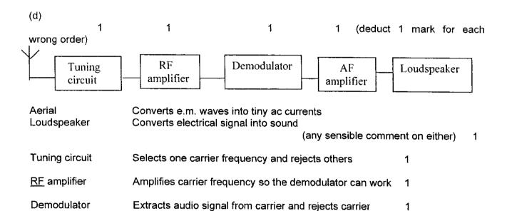
Amplifies audio signal to be able to drive loudspeaker
