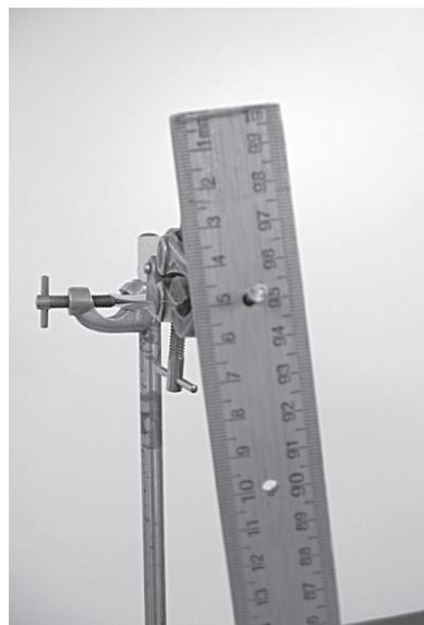
The rule is rotated through a small angle and released. It then oscillates about the pin as a pendulum with a time period  $T$ .
