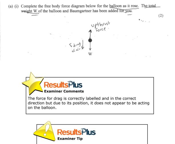
Free-body diagrams should show all the forces acting on a body with their correct directions. All lines with arrow heads must touch the dot to imply that the force is acting on the object the dot represents.
