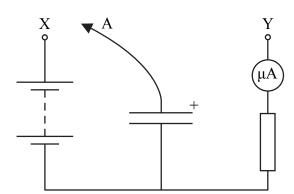
Use the spare lead to connect point X to point Y. Record the current  $I_0$ .
