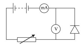
(b) Connect the battery and adjust the variable resistor until the current I is 5.0 mA. Record below the corresponding reading V on the voltmeter.
