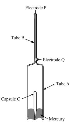
Radon gas,  $^{222}_{86}$  Rn , which decays by  $\alpha$ -emission to an isotope of polonium, Po, is placed at atmospheric pressure in a capsule C made from very thin glass. Any  $\alpha$ -particles passing through the glass from C become helium atoms in the evacuated tube A.
