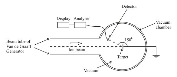
The RBS technique is illustrated above. Samples are mounted in a vacuum chamber which is connected to the beam tube of a Van de Graaff generator. This provides a mono-energetic beam of ions which strike the target sample. The particles backscattered through any particular angle, e.g. the 150° shown above, are detected and their energy is analysed. A typical incoming beam energy for helium ions is 2 MeV.
