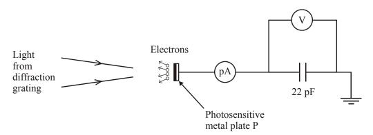
The picoammeter registers a current that falls gradually to zero when a certain wavelength of light is focused on P. At the same time the reading on the voltmeter rises from zero to a maximum of 0.58 V.
