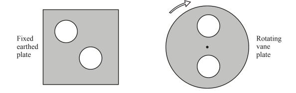
As the vane plate rotates, the Earth's electric field produces an induced charge on the vane plate and, by suitable connections to the plates, a small varying current can be detected. The peak value of this current can be found by passing the current through a resistor and measuring the resulting peak potential difference across the resistor.
