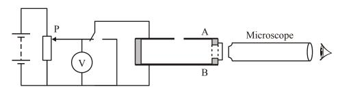
The action of spraying the oil causes the drops to become electrically charged. If now the plates are charged, the region between the plates becomes a uniform electric field, and by adjusting the potentiometer a drop can be held stationary between the plates. It can be shown that when the field has been adjusted to this value
