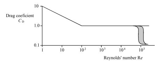
The graph shows how  $c_D$  varies with Re. The flat central section is where the drag is largely inertial and the sloping section where it is mostly viscous. The sudden drop at high values of Re is where the boundary layer (the liquid immediately in contact with the cylinder) becomes turbulent. The precise position of this transition depends on the roughness of the surface of the cylinder: a rough surface produces a lot of small-scale turbulence which hastens the transition.
