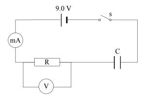
At t = 0 switch S is closed. Readings of the potential difference across the resistor are taken at regular intervals and the graph shown is obtained.
