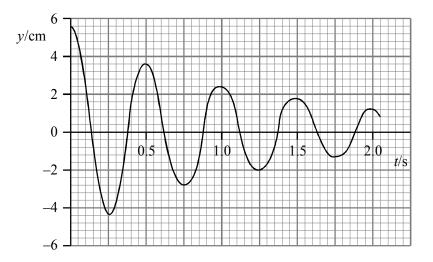
By taking measurements from the graph, discuss whether the damping is exponential in this case.
