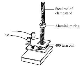
When there is an alternating current in the 400-turn coil, the aluminium ring rises to a few centimetres above the coil. Changes in the size of the alternating current make the ring rise to different heights.
