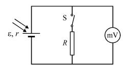
Explain how, by taking readings with the switch S first open and then closed, the student can find the value of *r*.
