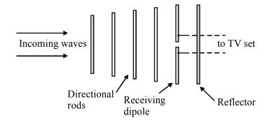
(i) The incoming signal is a plane polarised electromagnetic wave of frequency 1.07 GHz.
