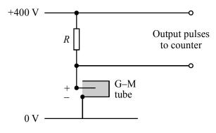
The G–M tube is connected in the circuit shown. When an ionizing particle enters the tube, the resulting pulse of current causes a corresponding pulse of p.d. across the resistance R in series with it. This is amplified and registered by a suitable device, e.g. a counter.
