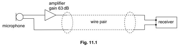
The microphone and amplifier are connected to a receiver by means of a wire pair having an attenuation of 12 dB per kilometre length. The output signal from the microphone is  $2.5 \,\mu\text{W}$  and there is a constant noise power in the wire pair of  $0.035 \,\mu\text{W}$ .
