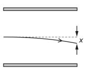
The vertical deflection *x* is measured at the right-hand edge of the plates.
