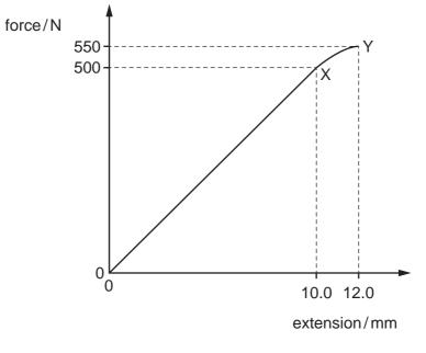
What is the total work done in stretching the sample from zero to 12.0 mm extension? Simplify the calculation by treating the curve XY as a straight line.
