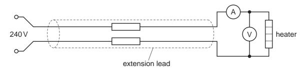
A voltmeter measures the potential difference (p.d.) across the heater as 216V and an ammeter measures the current through the heater as 7.7 A.
