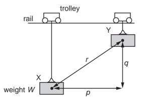
As a result, the weight moves through a distance r from X to Y. It starts and finishes at rest.
