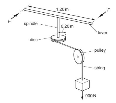
What is the minimum force *F*, applied to each end of the lever, that could lift the weight?
