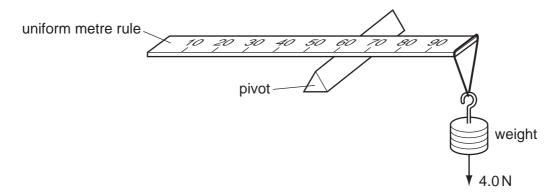
At the instant when the rule is horizontal, what is the resultant turning moment about the pivot?
