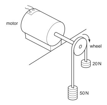
If the wheel is making 20 revolutions per second, what is the output power of the motor?
