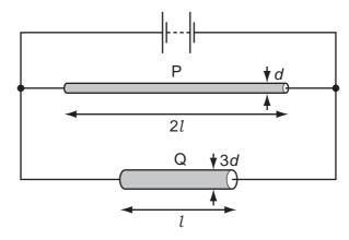
What is the ratio  $\frac{\text{current in P}}{\text{current in Q}}$ ?
