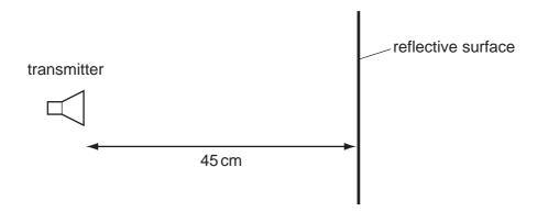
The emitted waves have a frequency of 1.00 GHz. A stationary wave is produced with a node at the transmitter and a node at the surface.
