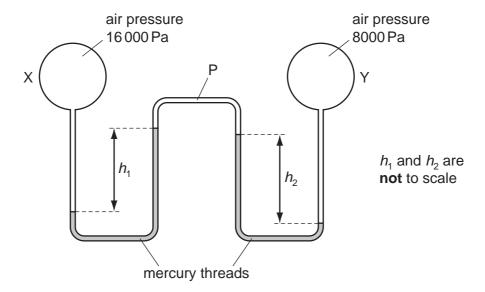
The density of mercury is 13 600 kg m<sup>-3</sup>.
