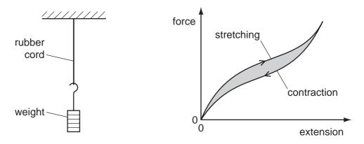
The force-extension curve for contraction is below the force-extension curve for stretching.
