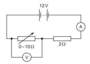
The resistance of the variable resistor is changed from zero to its maximum value.
