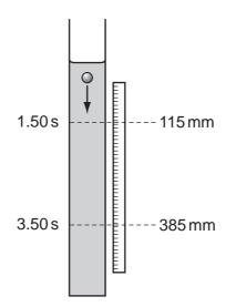
There are two marks on the tube. The top mark is positioned at  $115 \pm 1 \text{ mm}$  on the adjacent rule and the lower mark at  $385 \pm 1 \text{ mm}$ . The ball passes the top mark at  $1.50 \pm 0.02 \text{ s}$  and passes the lower mark at  $3.50 \pm 0.02 \text{ s}$ .
