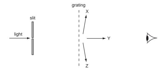
An observer views the slit through the grating at different angles, moving his head from X parallel to the grating, through Y, opposite the slit, to Z parallel to the grating on the opposite side.
