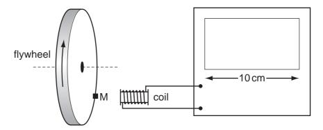
The flywheel has a small magnet M mounted on it. Each time the magnet passes the coil, a voltage pulse is generated, which is passed to the c.r.o. The display of the c.r.o. is 10 cm wide. The flywheel is rotating at a rate of about 3000 revolutions per minute.
