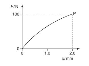
**20** The graph shows the non-linear force-extension curve for a wire made from a new composite material.
