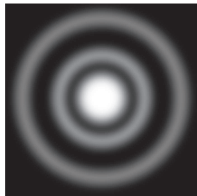
Fig. 10.2 Electron diffraction rings seen on the fluorescent screen
