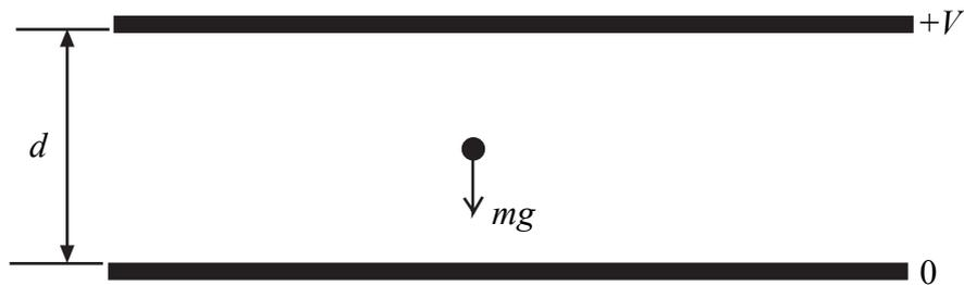
The diagram shows a charged oil drop of weight  $mg$ , which is stationary in the electric field between two parallel plates. If the potential difference between the plates is  $V$  and the separation of the plates is  $d$ , what is the charge on the oil drop?
