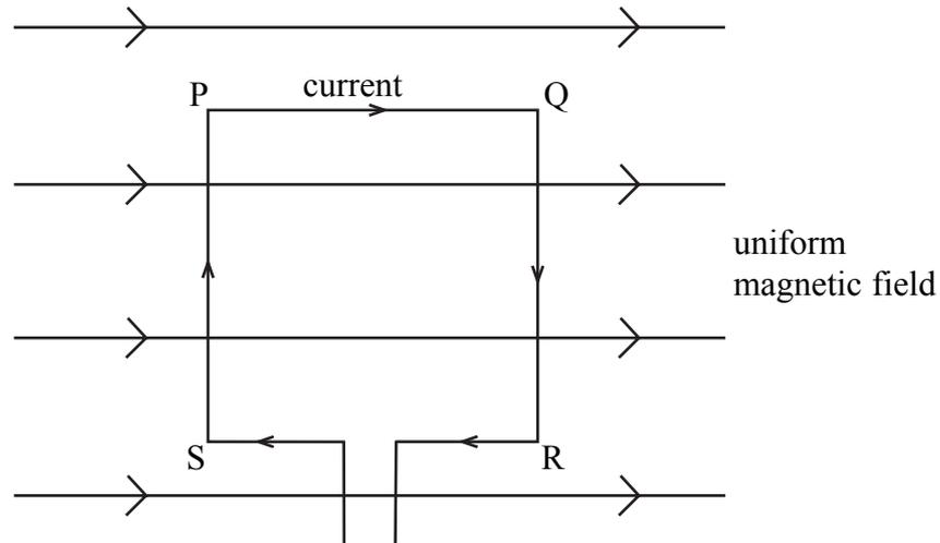
The diagram shows a square coil PQRS placed in a uniform magnetic field with the plane of the coil parallel to the lines of magnetic field. A constant current is passed round the coil in the direction shown, causing a force to act on side PS of the coil. Which one of the following statements about the forces acting on the other sides of the coil is correct?
