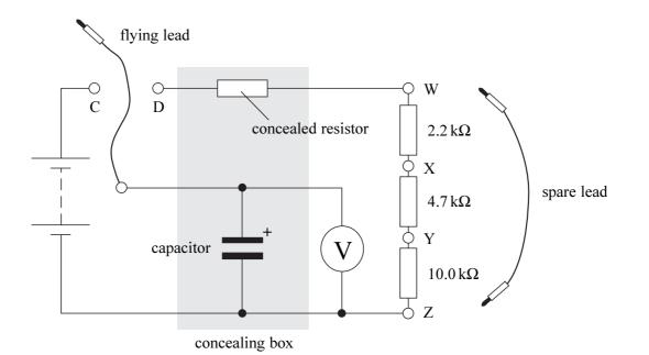
(a) With *R* set to zero resistance, charge the capacitor by connecting the flying lead to terminal C. The voltmeter will show a steady reading. Discharge the capacitor by connecting the flying lead to terminal D. The voltmeter reading will start to fall exponentially. Make suitable measurements to determine  $T_0$ , the time for the voltmeter reading to decrease by 50% when R = 0.
