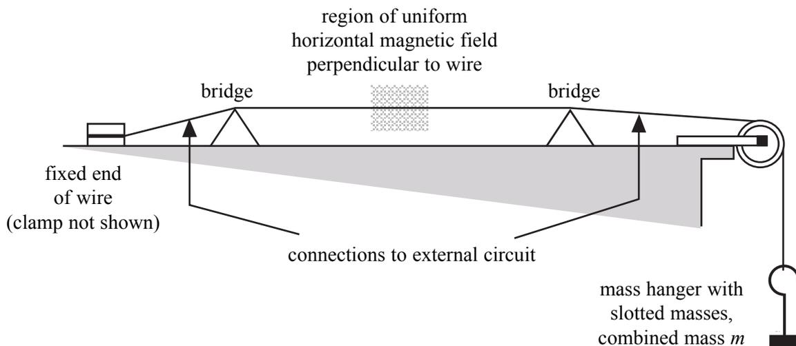
There is **no insistence** that the fixed end should be at the left-hand end of the arrangement as presented to the candidate. Note that each set will need to be set up parallel with, and close to, the edge of the bench, with the pulley overhanging the end of the bench. Ensure that the sections of the wire between bridge and fixed end, and between bridge and pulley, are not too steeply inclined, to enable ease of movement of the bridges.
