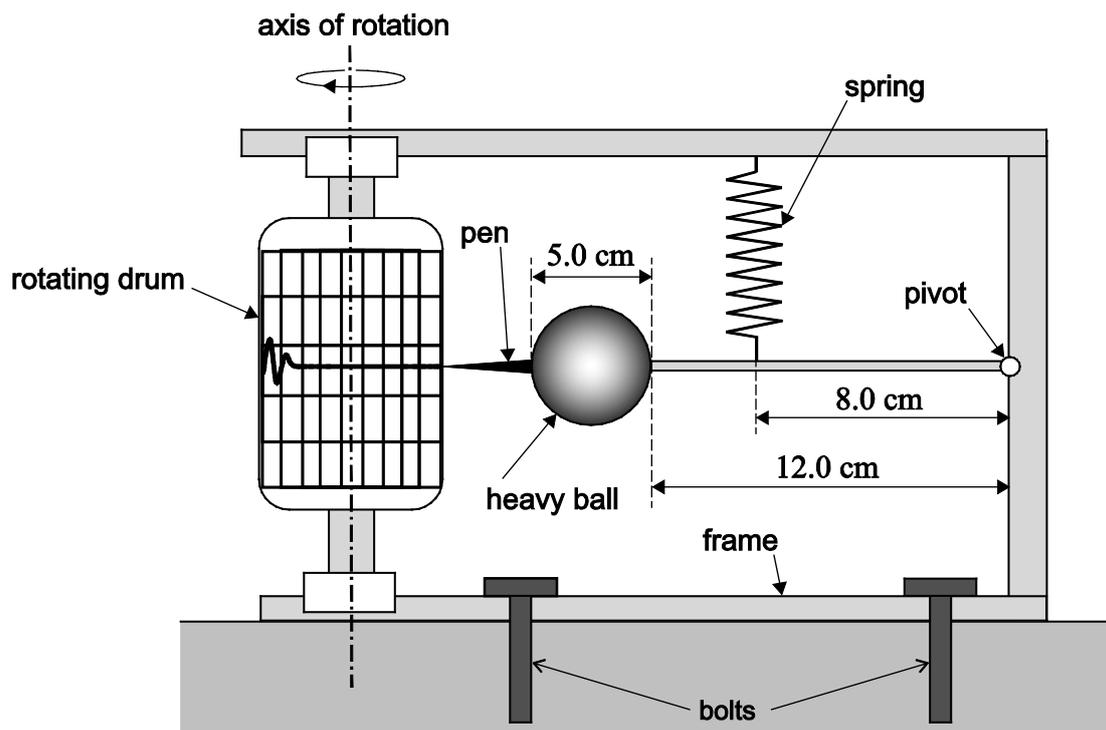
A heavy spherical ball is attached to a pivot by a rod so that the rod and ball can move in a vertical plane. The rod is suspended by a spring so that, in equilibrium, the spring is vertical and the rod is horizontal. A pen is attached to the ball. The pen draws a line on graph paper attached to a drum rotating about a vertical axis. Bolts secure the seismometer to the ground so that the frame of the seismometer moves during the earthquake.
