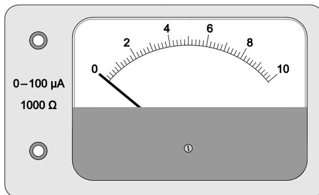
When this meter indicates a maximum reading and the needle points to the right-hand end of the scale (full-scale deflection), the current in the meter is  $100 \mu\text{A}$ . The meter has a resistance of  $1000 \Omega$ .
