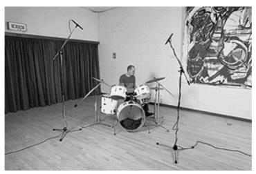
spaced overhead pair/stereo overhead pair to capture overall image/2m high large room/hard surfaces/no individual miking of drums
