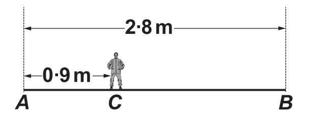
(a) Modelling the plank as a uniform rod, find the tensions in the ropes attached to the end A and the end B of the plank. [7]
