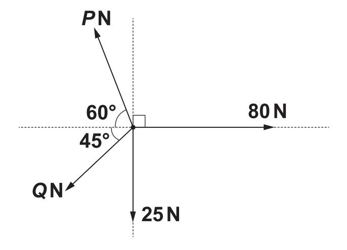
The diagram opposite shows four horizontal forces of magnitude PN, QN, 25N and 80N acting at a point.
