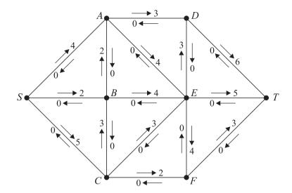
The diagram represents a system of pipes through which fluid can flow from a source, S, to a sink, T. The arrows are labelled to show excess capacities and potential backflows (how much more and how much less could flow in each pipe). The excess capacities and potential backflows are measured in litres per second. Currently no fluid is flowing through the system.
