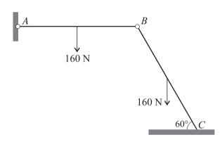
Two identical uniform rods, AB and BC, are freely jointed to each other at B, and A is freely jointed to a fixed point. The rods are in limiting equilibrium in a vertical plane, with C resting on a rough horizontal surface. AB is horizontal, and BC is inclined at  $60^{\circ}$  to the horizontal. The weight of each rod is 160 N (see diagram).
