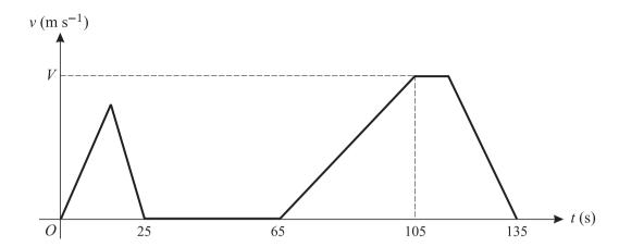
The diagram shows the (t, v) graph for the motion of a hoist used to deliver materials to different levels at a building site. The hoist moves vertically. The graph consists of straight line segments. In the first stage the hoist travels upwards from ground level for 25 s, coming to rest 8 m above ground level.
