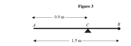
A uniform rod AB has length 1.5 m and mass 8 kg. A particle of mass m kg is attached to the rod at B. The rod is supported at the point C, where AC = 0.9 m, and the system is in equilibrium with AB horizontal, as shown in Figure 2.
