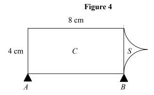
A tool is modelled as having two components, a solid uniform cylinder C and the solid S. The diameter of C is 4 cm and the length of C is 8 cm. One end of C coincides with the plane face of S. The components are made of different materials. The weight of C is 10W newtons and the weight of S is 2W newtons. The tool lies in equilibrium with its axis of symmetry horizontal on two smooth supports A and B, which are at the ends of the cylinder, as shown in Fig. 4.
