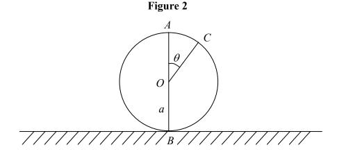
A particle is at the highest point *A* on the outer surface of a fixed smooth sphere of radius *a* and centre *O*. The lowest point *B* of the sphere is fixed to a horizontal plane. The particle is projected horizontally from *A* with speed *u*, where  $u < \sqrt{(ag)}$ . The particle leaves the sphere at the point *C*, where *OC* makes an angle  $\theta$  with the upward vertical, as shown in Fig. 2.
