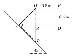
The diagram shows the cross-section OABCDE through the centre of mass of a uniform prism on a rough inclined plane. The portion ADEO is a rectangle in which  $AD = OE = 0.6 \,\mathrm{m}$  and  $DE = AO = 0.8 \,\mathrm{m}$ ; the portion BCD is an isosceles triangle in which angle BCD is a right angle, and A is the mid-point of BD. The plane is inclined at  $45^{\circ}$  to the horizontal, BC lies along a line of greatest slope of the plane and DE is horizontal.
