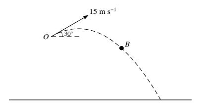
A small ball B is projected from a point O above horizontal ground, with initial speed  $15 \,\mathrm{m\,s^{-1}}$  at an angle of projection of 30° above the horizontal (see diagram). The ball strikes the ground 3 s after projection.
