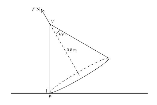
A uniform solid cone with height 0.8 m and semi-vertical angle  $30^{\circ}$  has weight 20 N. The cone rests in equilibrium with a single point *P* of its base in contact with a rough horizontal surface, and its vertex *V* vertically above *P*. Equilibrium is maintained by a force of magnitude *F* N acting along the axis of symmetry of the cone and applied to *V* (see diagram).
