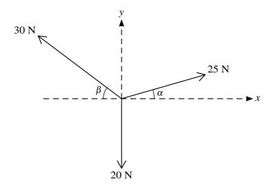
Three coplanar forces act at a point. The magnitudes of the forces are 20 N, 25 N and 30 N, and the directions in which the forces act are as shown in the diagram, where  $\sin \alpha = 0.28$  and  $\cos \alpha = 0.96$ , and  $\sin \beta = 0.6$  and  $\cos \beta = 0.8$ .
