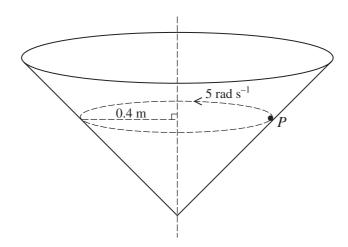
A particle P of mass 0.5 kg moves in a horizontal circle on the smooth inner surface of a hollow cone which is fixed with its axis vertical and its vertex downwards. P moves with angular speed 5 rad s<sup>-1</sup> in a circle of radius 0.4 m (see diagram). Show that the semi-vertical angle of the cone is 45° and calculate the magnitude of the force exerted on P by the surface of the cone. [6]
