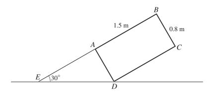
ABCD is the cross-section through the centre of mass of a uniform rectangular block of weight 260 N. The lengths AB and BC are 1.5 m and 0.8 m respectively. The block rests in equilibrium with the point D on a rough horizontal floor. Equilibrium is maintained by a light rope attached to the point A on the block and the point E on the floor. The points E, E0 and E1 lie in a straight line inclined at E30 to the horizontal (see diagram).
