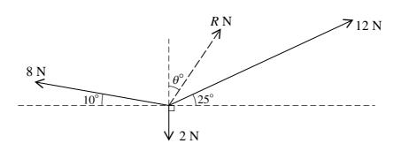
Three coplanar forces of magnitudes 8 N, 12 N and 2 N act at a point. The resultant of the forces has magnitude R N. The directions of the three forces and the resultant are shown in the diagram. Find R and  $\theta$ .
