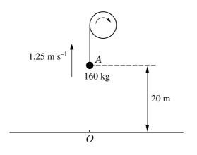
A load of mass 160 kg is pulled vertically upwards, from rest at a fixed point O on the ground, using a winding drum. The load passes through a point A, 20 m above O, with a speed of  $1.25 \text{ m s}^{-1}$  (see diagram). Find, for the motion from O to A,
