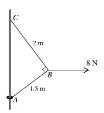
A small ring of mass 0.2 kg is threaded on a fixed vertical rod. The end A of a light inextensible string is attached to the ring. The other end C of the string is attached to a fixed point of the rod above A. A horizontal force of magnitude 8 N is applied to the point B of the string, where AB = 1.5 m and BC = 2 m. The system is in equilibrium with the string taut and AB at right angles to BC (see diagram).
