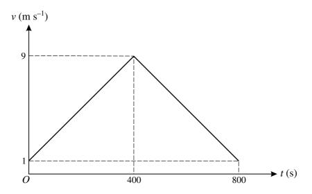
The diagram shows an approximate velocity-time graph for the motion of the tractor. The graph consists of two straight line segments. Use the graph to find an approximation for
