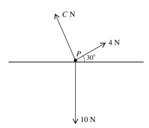
A particle P has weight  $10 \,\mathrm{N}$  and is in limiting equilibrium on a rough horizontal table. The forces shown in the diagram represent the weight of P, an applied force of magnitude  $4 \,\mathrm{N}$  acting on P in a direction at  $30^\circ$  above the horizontal, and the contact force exerted on P by the table (the resultant of the frictional and normal components) of magnitude  $C \,\mathrm{N}$ .
