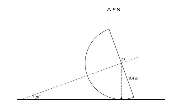
A smooth hemispherical shell, with centre O, weight 12 N and radius 0.4 m, rests on a horizontal plane. A particle of weight W N lies at rest on the inner surface of the hemisphere vertically below O. A force of magnitude F N acting vertically upwards is applied to the highest point of the hemisphere, which is in equilibrium with its axis of symmetry inclined at 20° to the horizontal (see diagram).
