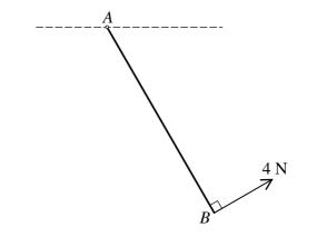
A uniform rod AB of weight 16 N is freely hinged at A to a fixed point. A force of magnitude 4 N acting perpendicular to the rod is applied at B (see diagram). Given that the rod is in equilibrium,
