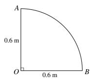
AOB is a uniform lamina in the shape of a quadrant of a circle with centre O and radius  $0.6\,\mathrm{m}$  (see diagram).
