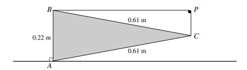
ABC is a uniform triangular lamina of weight 19 N, with AB = 0.22 m and AC = BC = 0.61 m. The plane of the lamina is vertical. A rests on a rough horizontal surface, and AB is vertical. The equilibrium of the lamina is maintained by a light elastic string of natural length 0.7 m which passes over a small smooth peg P and is attached to B and C. The portion of the string attached to B is horizontal, and the portion of the string attached to C is vertical (see diagram).
