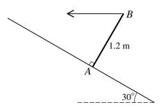
A uniform rod AB has weight 15 N and length 1.2 m. The end A of the rod is in contact with a rough plane inclined at 30° to the horizontal, and the rod is perpendicular to the plane. The rod is held in equilibrium in this position by means of a horizontal force applied at B, acting in the vertical plane containing the rod (see diagram).
