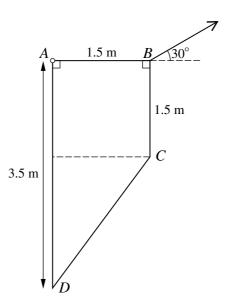
A uniform lamina of weight 15 N is in the form of a trapezium ABCD with dimensions as shown in the diagram. The lamina is freely hinged at A to a fixed point. One end of a light inextensible string is attached to the lamina at B. The lamina is in equilibrium with AB horizontal; the string is taut and in the same vertical plane as the lamina, and makes an angle of  $30^{\circ}$  upwards from the horizontal (see diagram). Find the tension in the string.
