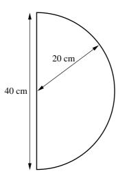
A frame consists of a uniform semicircular wire of radius 20 cm and mass 2 kg, and a uniform straight wire of length 40 cm and mass 0.9 kg. The ends of the semicircular wire are attached to the ends of the straight wire (see diagram). Find the distance of the centre of mass of the frame from the straight wire.
