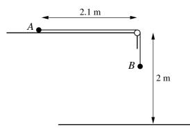
Particles A and B, of masses 0.2 kg and 0.45 kg respectively, are connected by a light inextensible string of length 2.8 m. The string passes over a small smooth pulley at the edge of a rough horizontal surface, which is 2 m above the floor. Particle A is held in contact with the surface at a distance of 2.1 m from the pulley and particle B hangs freely (see diagram). The coefficient of friction between A and the surface is 0.3. Particle A is released and the system begins to move.
