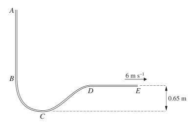
A smooth narrow tube AE has two straight parts, AB and DE, and a curved part BCD. The part AB is vertical with A above B, and DE is horizontal. C is the lowest point of the tube and is 0.65 m below the level of DE. A particle is released from rest at A and travels through the tube, leaving it at E with speed  $6 \,\mathrm{m\,s^{-1}}$  (see diagram). Find
