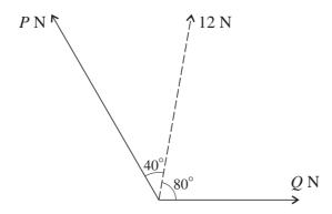
Two forces have magnitudes PN and QN. The resultant of the two forces has magnitude 12N and acts in a direction  $40^{\circ}$  clockwise from the force of magnitude PN and  $80^{\circ}$  anticlockwise from the force of magnitude QN (see diagram). Find the value of Q.
