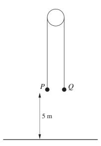
Particles P and Q, of masses  $0.55\,\mathrm{kg}$  and  $0.45\,\mathrm{kg}$  respectively, are attached to the ends of a light inextensible string which passes over a smooth fixed pulley. The particles are held at rest with the string taut and its straight parts vertical. Both particles are at a height of 5 m above the ground (see diagram). The system is released.
