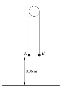
Particles A and B are attached to the ends of a light inextensible string which passes over a smooth pulley. The system is held at rest with the string taut and its straight parts vertical. Both particles are at a height of  $0.36 \,\mathrm{m}$  above the floor (see diagram). The system is released and A begins to fall, reaching the floor after  $0.6 \,\mathrm{s}$ .
