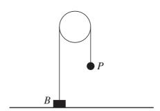
A block B of mass 5 kg is attached to one end of a light inextensible string. A particle P of mass 4 kg is attached to other end of the string. The string passes over a smooth pulley. The system is in equilibrium with the string taut and its straight parts vertical. B is at rest on the ground (see diagram). State the tension in the string and find the force exerted on B by the ground. [3]
