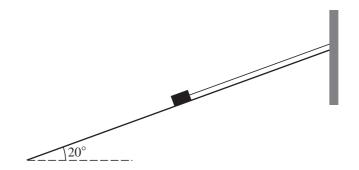
A block of mass 8 kg is at rest on a plane inclined at  $20^{\circ}$  to the horizontal. The block is connected to a vertical wall at the top of the plane by a string. The string is taut and parallel to a line of greatest slope of the plane (see diagram).
